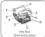
A=WIRE BLADE **B=WIRE GROOVE** C=STRIP HOLDER D=STRIP END PIN **E=BASE SIDE LATCH** F=CAP LATCH HOLE G=CAP PRESSING BAR
